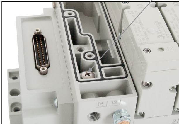
Internal Pilot Supply Plug Location
